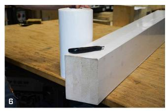
DEFENCE REMOVABLE should also be applied to the beam's end grain, particularly during transport, to protect the timber from accidental damage.
