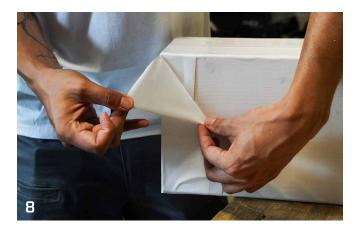
Remove DEFENCE ADHESIVE REMOVABLE. Within 8 weeks if exposed directly to weathering and UV rays.
